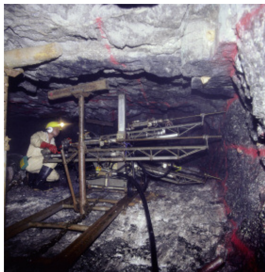
Deep-level mining of pgms on South Africa’s Bushveld Igneous Complex presents many challenges. The relative density of the host rock is greater than that generally associated with gold mines on the Witwatersrand complex, so rock pressures and associated seismicity increase with depth at a higher rate. Ambient mining temperatures also increase much faster. Photo courtesy Northam Platinum Limited; all other photos courtesy Heraeus
