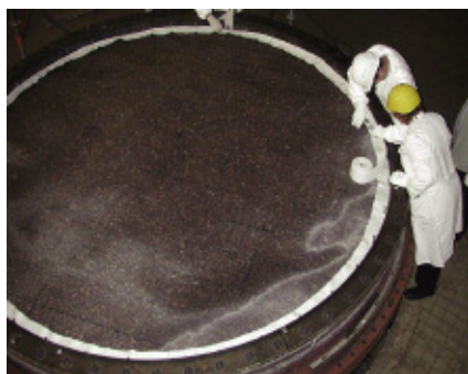
Gauze made of a platinum/rhodium alloy, used to produce nitric acid for the fertiliser industry.
