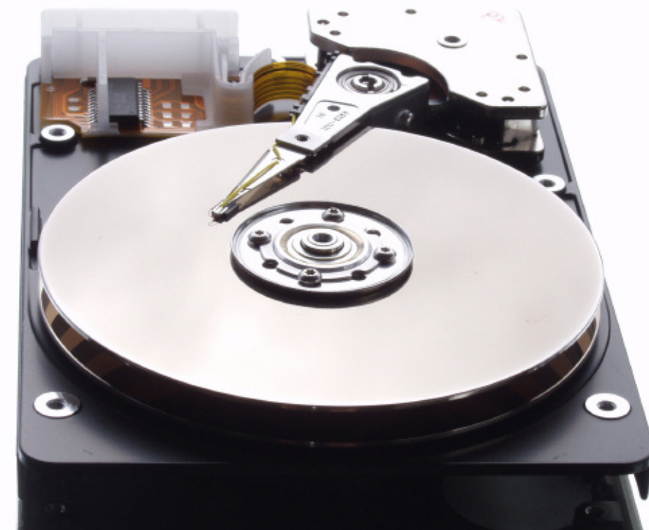
Hard disk drives are coated with a total of up to 16 different layers, four of them containing ruthenium.
